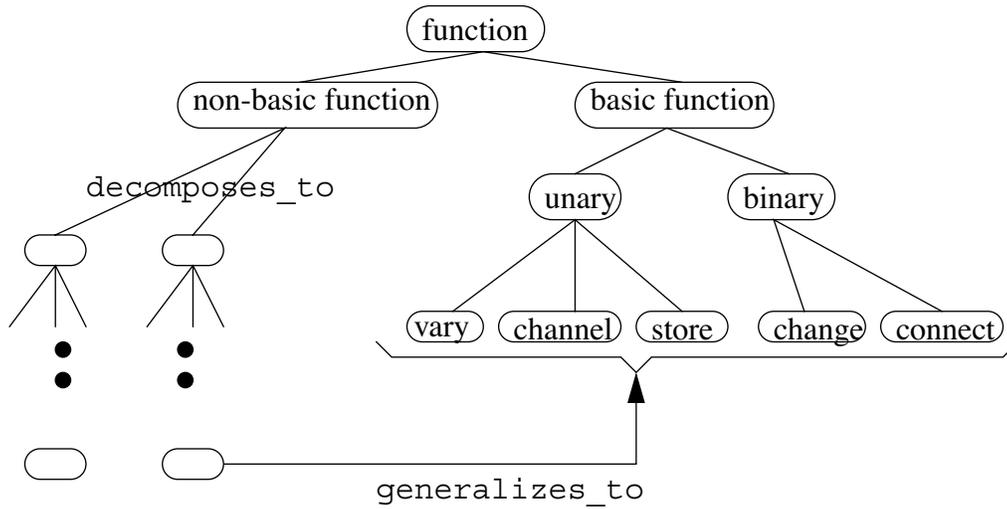
The aim of the function representation reported in (Pahl and Beitz, 1988) is to aid the novice designer in the design process. The design process is envisioned as guided by the functions and their decompositions (the so called function structures).
