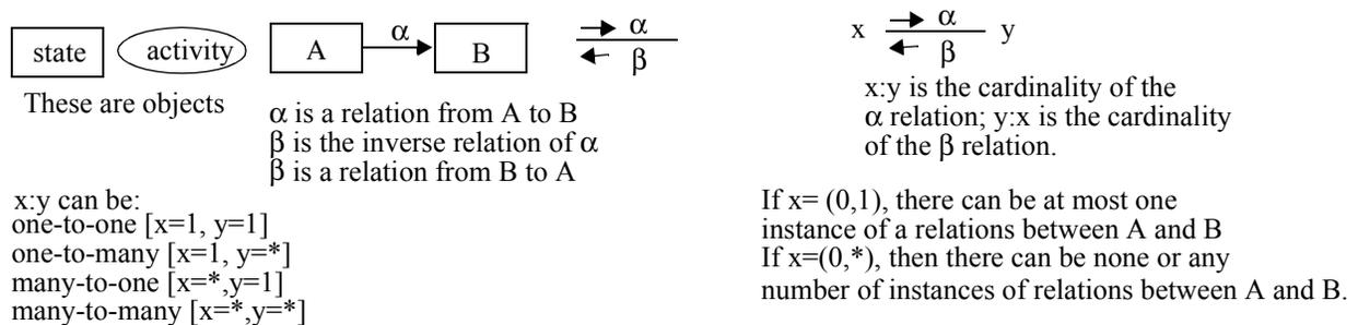
The fundamental data model for the Core Ontologies is called the activity cluster, and is shown below. At a given point in time, the modelled world is in one situation but activities and resources modelled with activity clusters can be in many states. When there is a state change to a resource or activity of an activity cluster, the situation of the modelled world changes.
