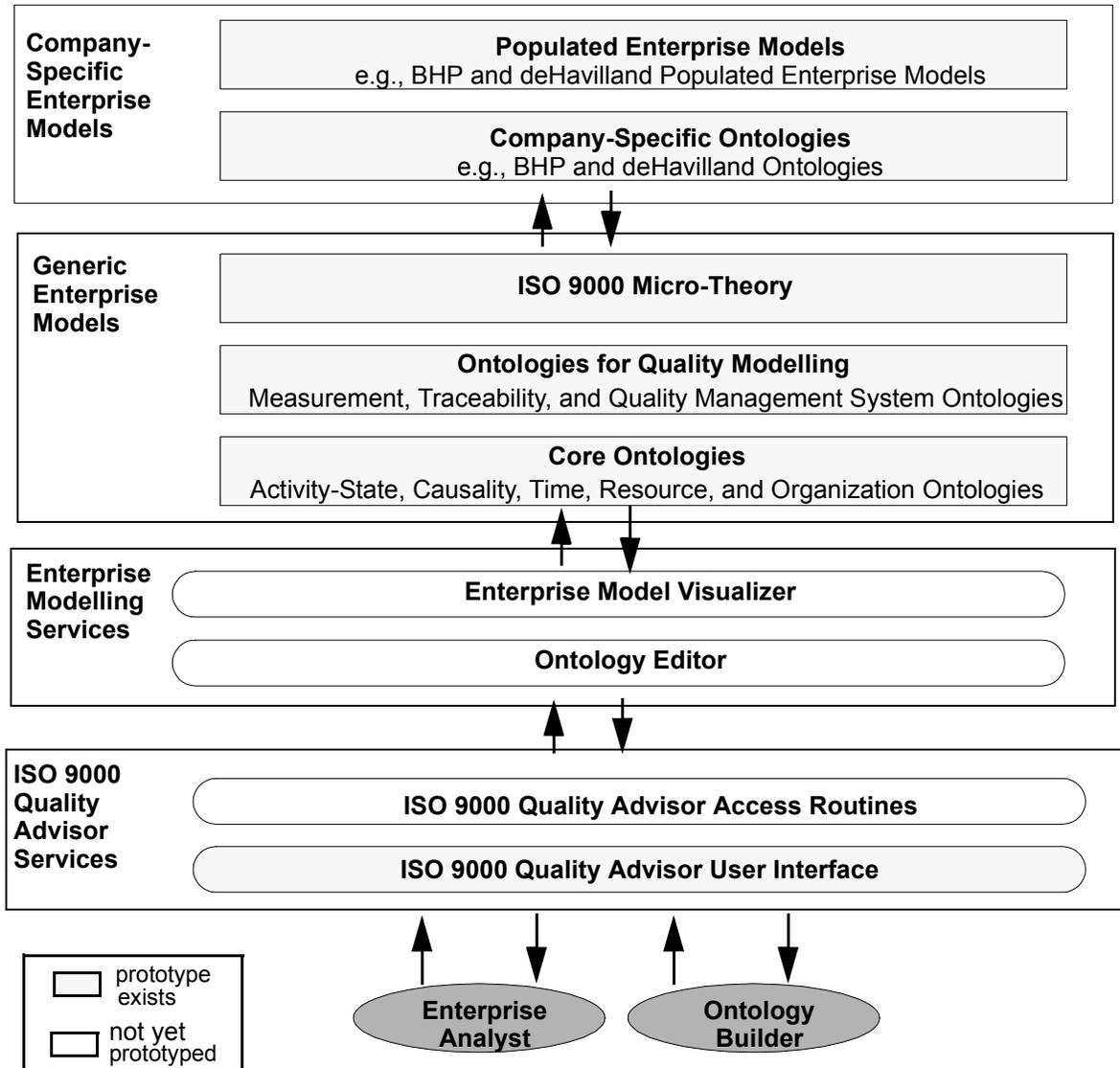
The front-end of the advisor is of an html user interface which access routines that enable the user to query populated enterprise models that are constructed upon generic models. The access routines also enable the user to access information system services that allow model visualization and editing. Below, the components of the architecture are described.
